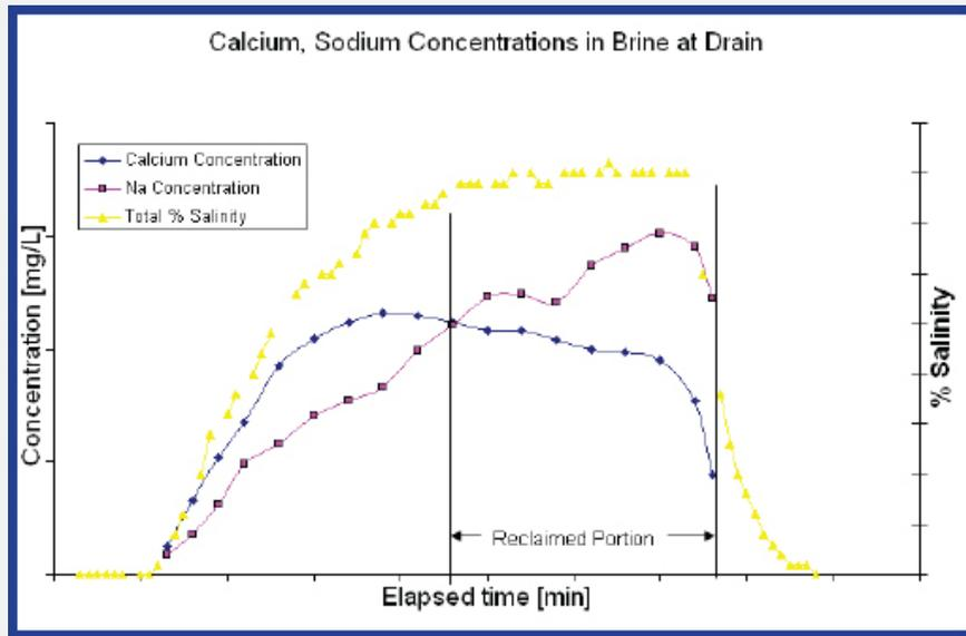
A system was set up in Pentair's water lab to test the efficacy of brine recovery. Brine was diverted from the drain at the peak of sodium concentration and sent back to the brine tank. The majority of the brine is made up from reclaim, except for enough fresh water to dissolve 2 pounds of salt. After regeneration, the total salt dissolved from the brine tank was recorded and plotted against the measured capacity.
