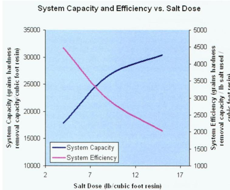
As shown above, the capacity of a softener will increase as the salt dose increases. However, it is also shown that brine efficiency decreases as the salt dose is increased because less capacity is gained for each additional pound of salt used. For example, 4 pounds of salt gives a capacity of 17,900 grains. Increasing the salt dose to 9 pounds of salt increases the salt used by a factor of 2.25, while capacity only increases to 26,600 grains, an increase of 1.5 times.
