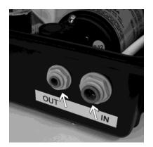
3. Connect the tubing that comes with the SDI-2000 unit from the pump "OUT" Port to the "IN" port on the SDI-2000 unit. Connect the filter holder (without a filter) to the "OUT" port on the SDI test kit, and position the filter holder over a drain.
