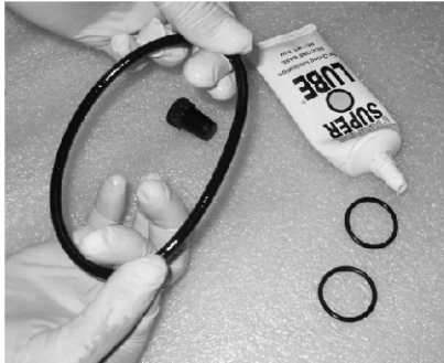
Lubricating Plug seals and O-rings
