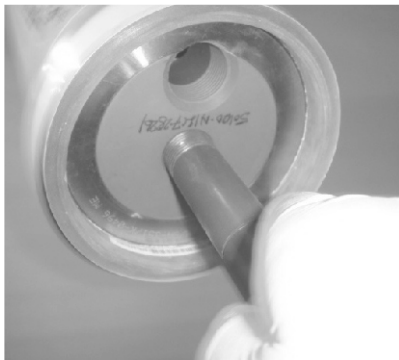
Removal of Head Assembly
