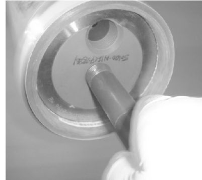
Installation of the End Plug Assembly into the vessel
