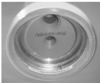
Retaining ring seated in the groove
