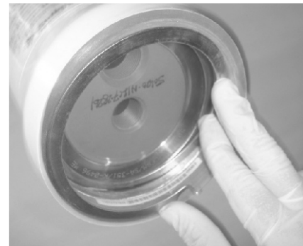
Inserting Retaining Ring into the groove
