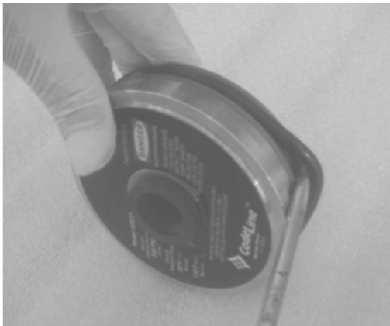
Removal of the Head Seal
