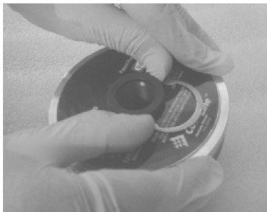
Removal of the Port Retainer Ring
