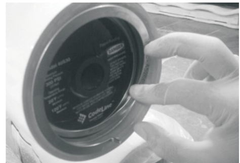
Inserting Retaining Ring into the groove
