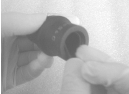
Inserting PWT / Adapter Seal
