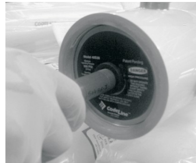
Removing the head assembly
