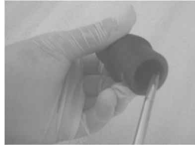
Removal of the PWT/Adapter Seal
