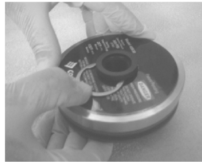
Installing Port Retainer
