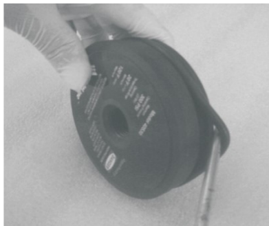
Removal of the Head Seal
