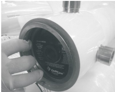
Removal of Retaining Ring
