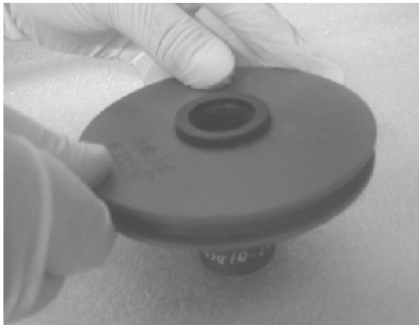
Installing Sealing Plate
