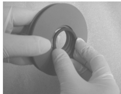
Inserting Permeate Port seal
