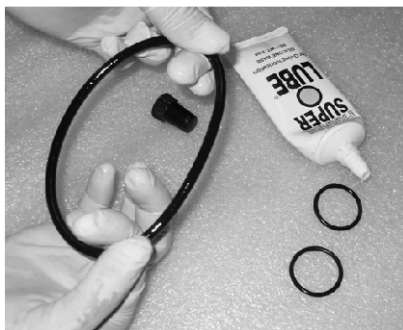
Lubricating Plug seals and O-rings
