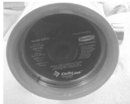
Retaining ring seated in the groove
