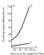
Curve B shows the starting and stop height differential of the Kari Float Switch in relationship to the distance of the weight from the float. Curve C shows the equivalent differential between starting and alarm levels. For example: On type 3H, if distance of the weight from float (A) is about 50 cm, then the start / stop differential is about 50 cm and the start / alarm differential is about 12 cm.
