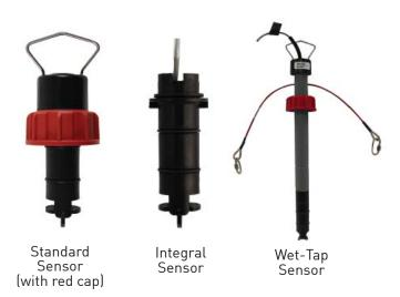
Simple to install with time-honored reliable performance, Signet 515 Rotor-X Paddlewheel Flow Sensors are highly repeatable, rugged sensors that offer exceptional value with little or no maintenance. The output signal of the Model 515 is a sinusoidal frequency capable of driving a self-powered flowmeter (Model 3-5090). The wide dynamic flow range of 0.3 to 6 m/s (1 to 20 ft/s) allows the sensor to measure liquid flow rates in full pipes and can be used in low pressure systems.
