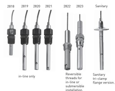
Signet 2818-2823 Conductivity/Resistivity Electrodes are designed to provide versatile installation and accurate sensing across a very broad dynamic range. These electrodes are built with a controlled surface finish to ensure accuracy and repeatability. The standard electrode is constructed 316 SS or Titanium, but there are other materials available for maximum chemical compatibility.
