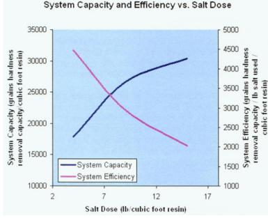
As shown above, the capacity of a softener will increase as the salt does increases. However, it is also shown that brine efficiency decreases as the salt dose is increased because less capacity is gained for each additional pound of salt used. For example, 4 pounds of salt gives a capacity of 17,900 grains. Increasing the salt dose to 9 pounds of salt increases the salt used by a factor of 2.25, while capacity only increases to 26,600 grains, an increase of 1.5 times.
