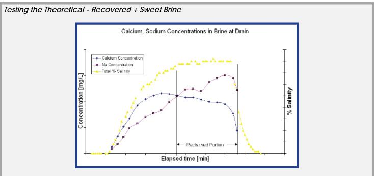
A system was set up in Pentair's water lab to test the efficacy of brine recovery. Brine was diverted from the drain at the peak of sodium concentration and sent back to the brine tank. The majority of the brine is made up from reclaim, except for enough fresh water to dissolve 2 pounds of salt. After regeneration, the total salt dissolved from the brine tank was recorded and plotted against the measured capacity.
