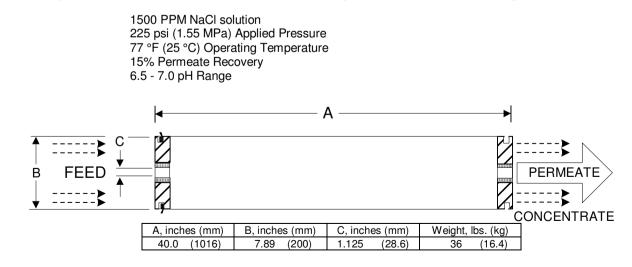
Notice: Permeate flow for individual elements may vary ±15 percent. Membrane active area may vary +/-4%. All membrane elements are supplied with a brine seal, interconnector, and o-rings. Elements are vacuum sealed in a polyethylene bag containing less than 1.0% sodium meta-bisulfite solution, and then packaged in a cardboard box.
