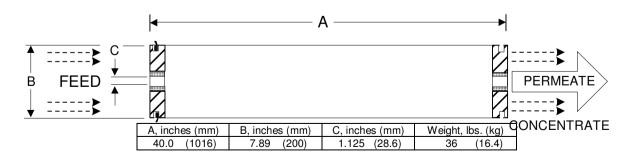
Notice: Permeate flow for individual elements may vary + 25 or - 15 percent. All membrane elements are supplied with a brine seal, interconnector, and o-rings. Elements are enclosed in a sealed polyethylene bag containing less than 1.0% sodium meta-bisulfite solution and 10% propylene glycol, and then packaged in a cardboard box.
