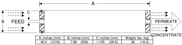
**Notice:** Permeate flow for individual elements may vary + or - 15 percent. Membrane active area may vary +/-4%. All membrane elements are supplied with a brine seal, interconnector, and o-rings. Elements are enclosed in a sealed polyethylene bag containing less than 1.0% sodium meta-bisulfite solution, and then packaged in a cardboard box.
