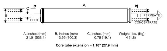
Notice: Minimum permeate flow for individual elements is 15 percent below listed flow. All membrane elements are supplied with a brine seal and o-rings. Most elements are packaged dry, sealed in a polyethylene bags, and shipped in a cardboard box. Some elements are sealed in polyethylene bags containing less than 1.0% sodium meta-bisulfite solution and shipped in a cardboard box.
