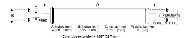
Notice: Permeate flow for individual elements may vary + or - 20 percent. All membrane elements are supplied with a brine seal, interconnector, and orings. Elements are vacuum-sealed in a polyethylene bag containing less than 1.0% sodium meta-bisulfite solution, and then packaged in a cardboard box.
