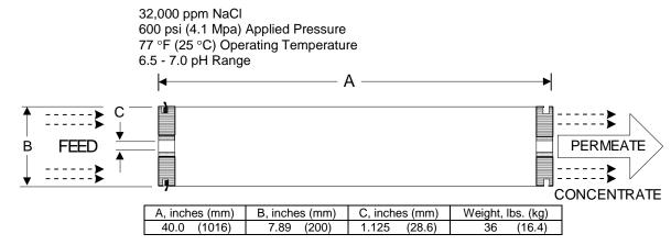
Permeate flow for individual elements may vary +25% or -15%. Membrane active area may vary +/-4%. All membrane elements are supplied with a brine seal, Notice: interconnector, and o-rings. Elements are vacuum sealed in a polyethylene bag containing less than 1.0% sodium meta-bisulfite solution, and then packaged in a cardboard box
