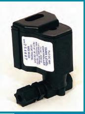
Our TLC Series utilizes a switch/valve combination which automatically shuts off feed water at a predetermined "full level" and then reopens the integral feed water valve at a second "refill level". The TLC Series provides a switched output to control a pump or other accessory.
