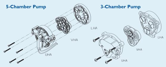
**UHA:** Upper Housing Assembly • **VHA:** Valve Housing Assembly • **LHA:** Lower Housing Assembly Distributed by Applied Membranes, Inc. | www.appliedmembranes.com | (760) 727-3711 | USA
