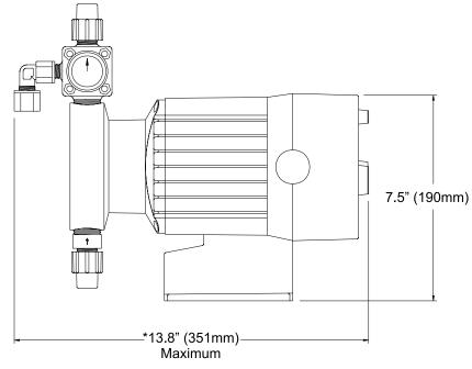
\*Dimensions shown are maximum for largest liquid end available.These dimensions vary depending on the liquid end selected.
