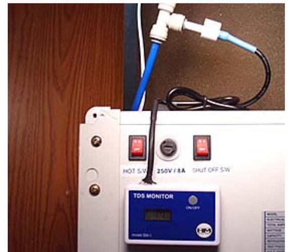
*Use the monitor to determine when a filter need to be changed.*
