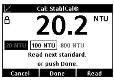
In the full calibration mode (0 to 1000 NTU), the text-based, assisted calibration feature walks you through clear and easy steps, and verifies the accuracy of your calibration automatically. This on-screen assistance eliminates the need for a manual and provides assurance that your calibration is complete and valid.
