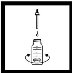
5. If the sample turns pink, add Sulfuric Acid Standard Solution one drop at a time. Count each drop. Swirl the mixing bottle after each drop is added. Add drops until the sample turns colorless.
