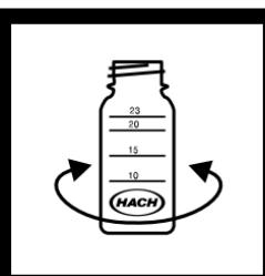
3. Swirl to mix. If the sample remains colorless, the phenolphthalein alkalinity is zero. In this case, proceed to Step 6.
