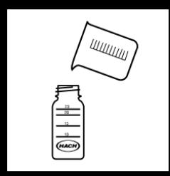
1. Fill the mixing bottle to the 23-mL mark with the sample water.
