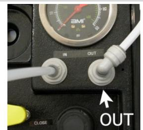
4. Once all connections are made, direct the outlet from the (empty) filter holder to drain. Turn the feed water on by turning the control valve handle counter-clockwise to the open position. Allow the system to run for approximately 15 seconds to flush and purge the air from the system.
