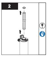
Remove the quartz sleeve from the UV chamber.
