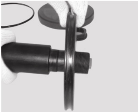
Installing Sealing Plate
