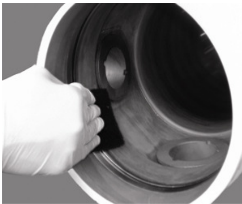
Cleaning inside the vessel
