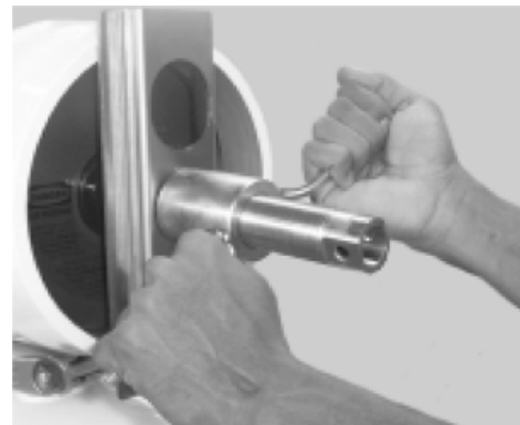
Removing Head Assembly using Head Removal Tool
