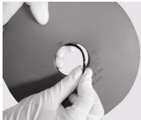
Installing Permeate Port Seal
