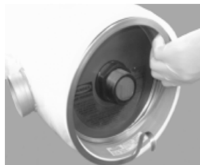
Removing the retaining ring from the groove
