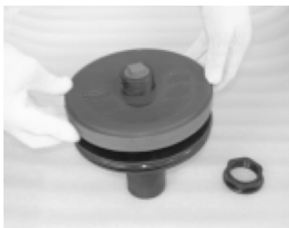
Removing the Bearing Plate
