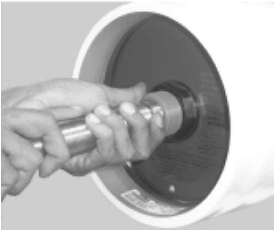
Removing Head Assembly
