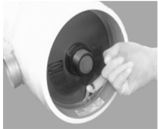
Lifting end of retaining ring out of groove
