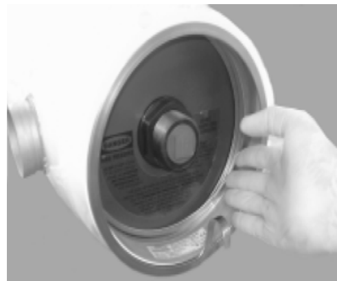
Installing Head Retaining ring
