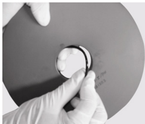
Installing Permeate Port Seal
