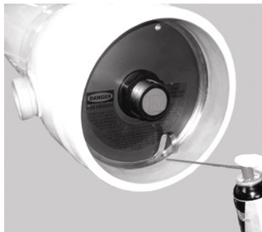
Applying penetrating fluid
