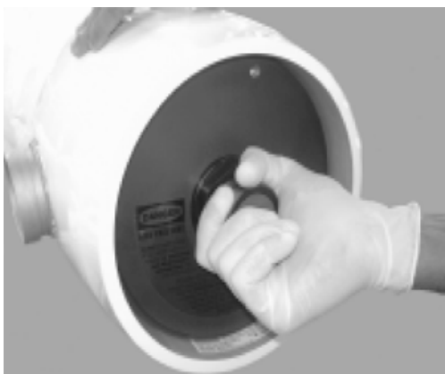
Installing Head Assembly
