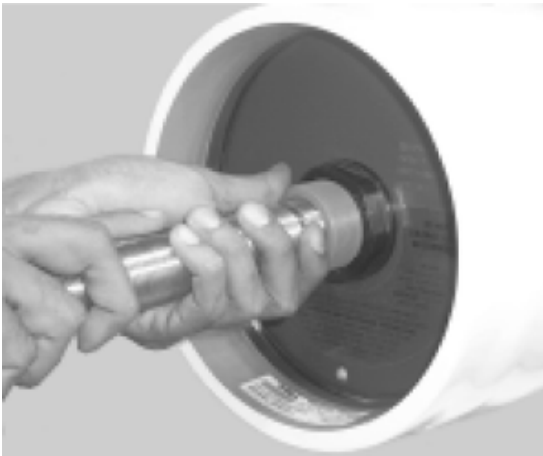
Removing Head Assembly
