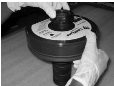
Removing the Permeate Port
