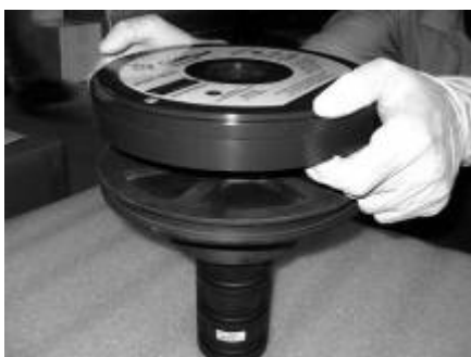
Removing the Bearing Plate
