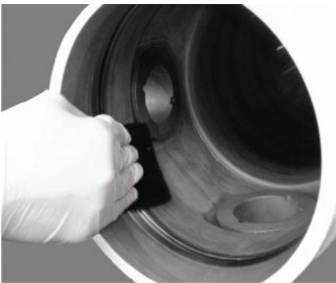
Cleaning inside the vessel
