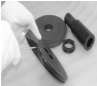
Removing the Head Seal
