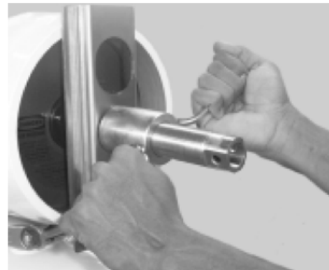
Removing Head Assembly using Head Removal Tool
