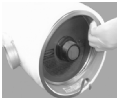
Removing the retaining ring from the groove
