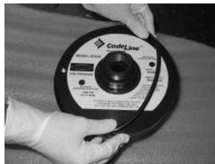
Installing Head Seal
