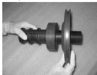
Removing the Sealing Plate
